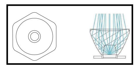
[ Using high efficiency total reflection lens ]
