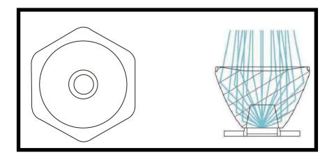
[Using high efficiency total reflection lens]
