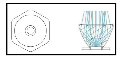
[ Using high efficiency total reflection lens ]
